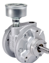
Model 6AM Up to 4 HP Speeds: 300-3,000 rpm Max. pressure 100 psi (7 bar)
